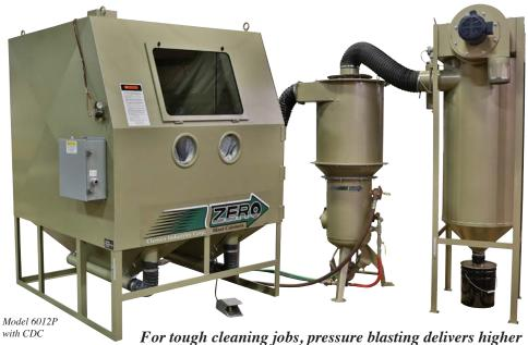
abrasive velocity for greater impact intensity, compared to suction blasting, and can increase your production rate by as much as 300 percent.
