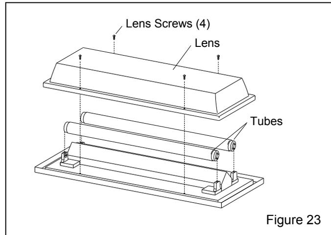
**7.7.3.3** Remove the four lens screws and remove the lens.
