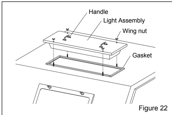
**7.7.2.2** Remove all the old gasket material and clean the surfaces of the cabinet.
