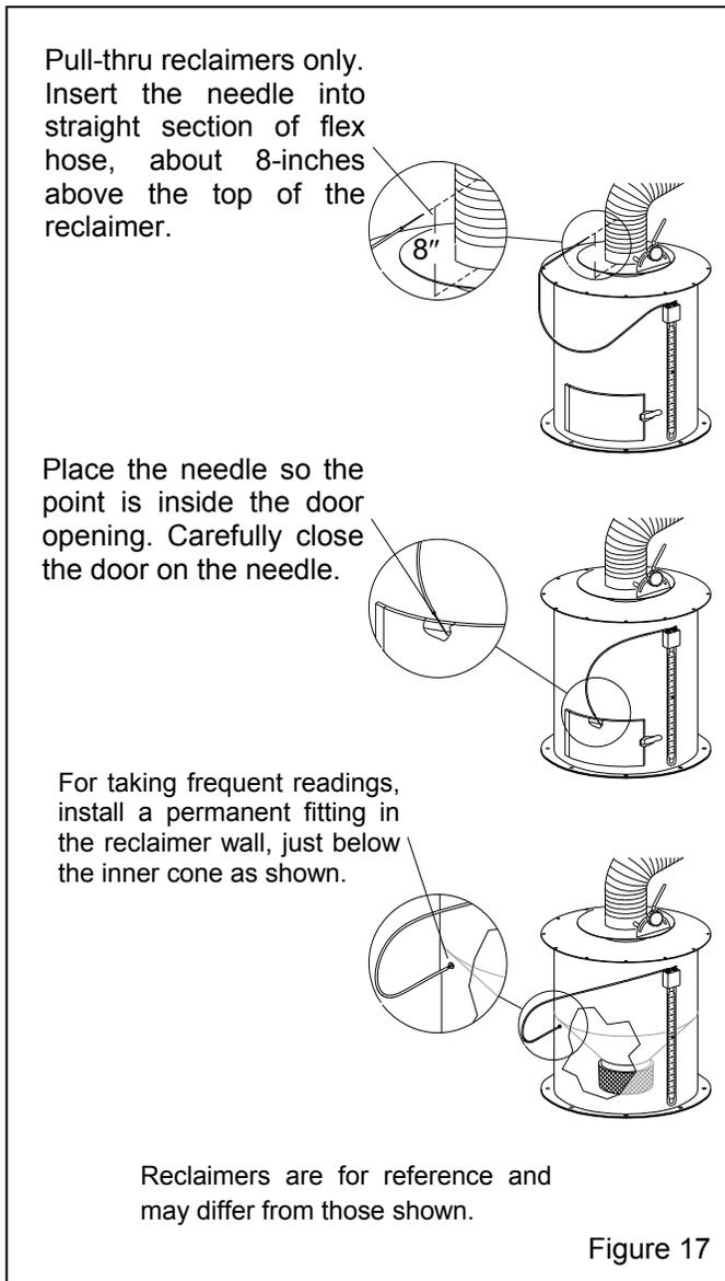
**5.7.8** Turn the exhauster ON. The negative (static) pressure will move fluid in the tube.
