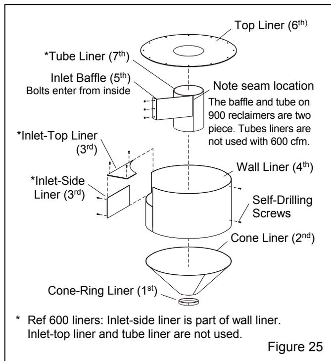
**7.11.12 (3<sup>rd</sup>)** Position the inlet-side liner and inlet-top liner to make sure they fit; trimming is occasionally required. Align the inlet-side liner and inlet-top liner and clamp them in place. Use a self-drilling screw at each hole location in the weldment to secure replacement liners. NOTE: To field install new, first-time inlet-side liner and inlet-top liners, after clamping the liners, use self-drilling screws at each liner corner to secure them.
