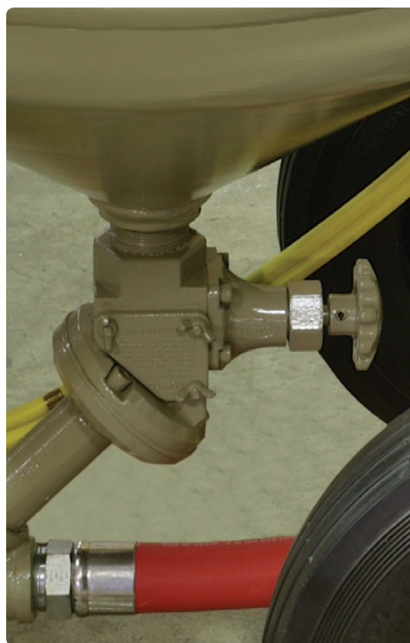
The Quantum Metering Valve features precision adjustment.
