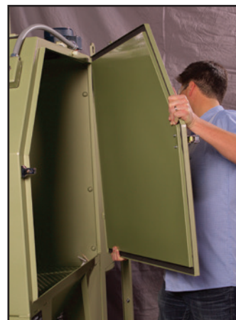
Lift-off hinges let you remove and replace the door in seconds, without tools.
