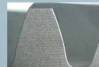
Tooth flanks, finished
