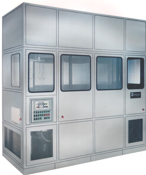
Sonicator CUDR-120 Vapor Degreaser With Sonicator "RCT" Automation/Process Control System, and full system Enclosure
