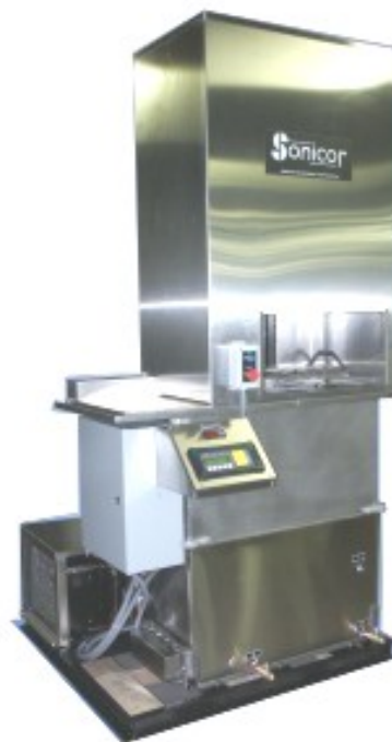
Sonicator UDR-70 Vapor Degreaser With Sonicator "VWE" Vertical Workload Elevator, and stainless upper enclosure
