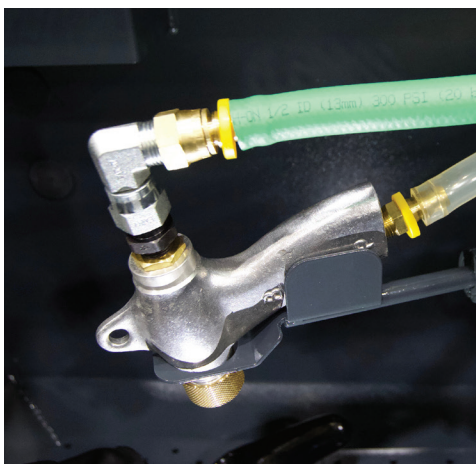
The BNP Blast Gun is height and angle adjustable, and also can be detached and handheld.
